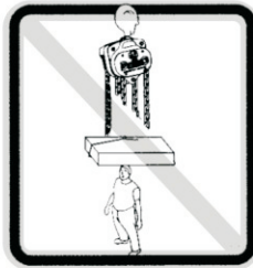
DO NOT allow anyone to stand or pass beneath the raised load
