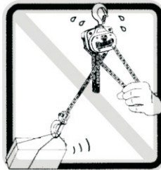
DO NOT use the chain block to drag the load across the floor
